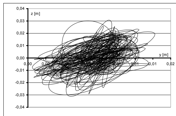
Figure 10. Planar motion of the central point of span of Tylmanowa footbridge.
