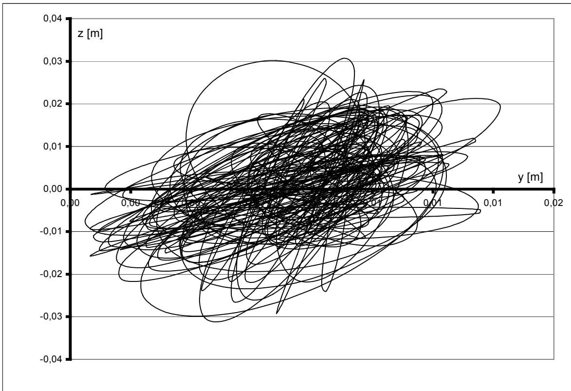
Fig. 15. Planar motion of the central point of span of the Tylmanowa footbridge.
