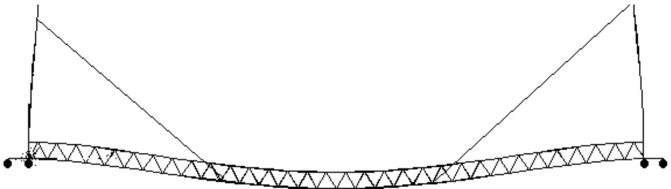
Fig. 14. II-nd symmetrical vibration mode of Footbridge D, side view
