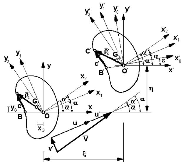
Fig. 1 Systems of coordinates and relations between different geometrical quantities in the case of a moving structure and an unsteady air onflow
