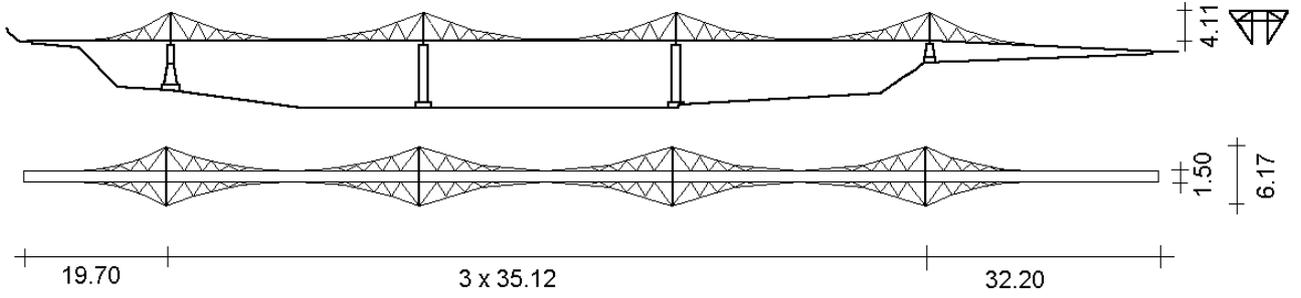
Fig. 4. View of footbridge B in Rożnów (dimension in meters)
