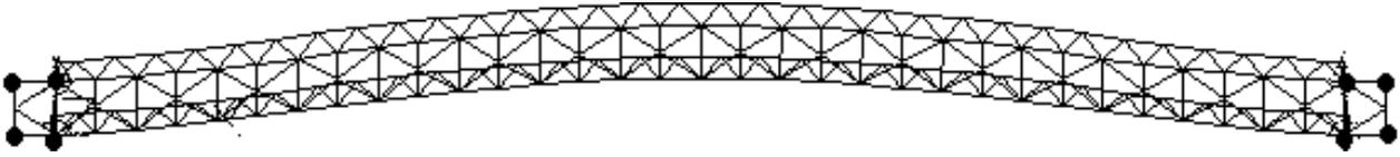
Fig. 13. I-st symmetrical vibration mode of footbridge D, plain view
