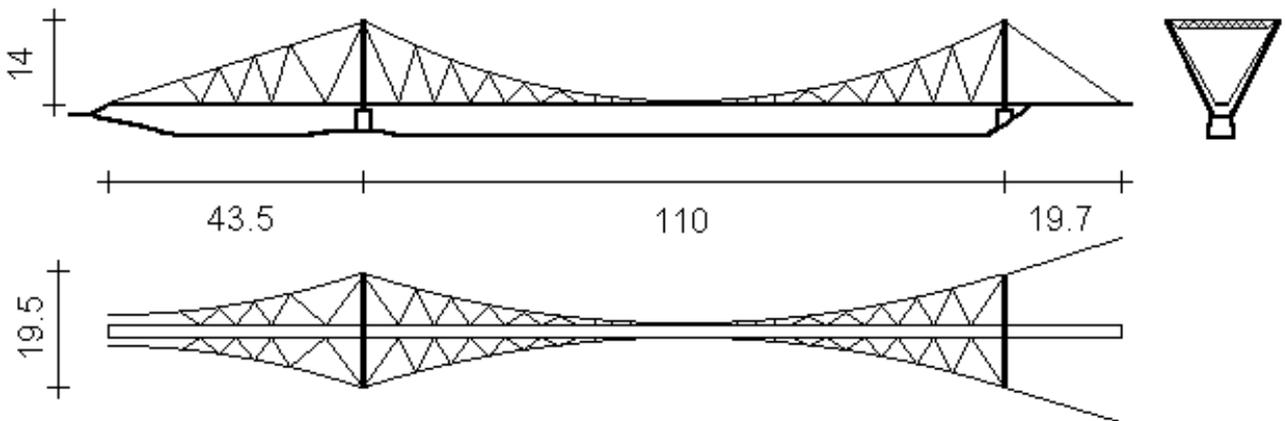
Fig. 5 View of footbridge C in Tropie (dimension in meters)
