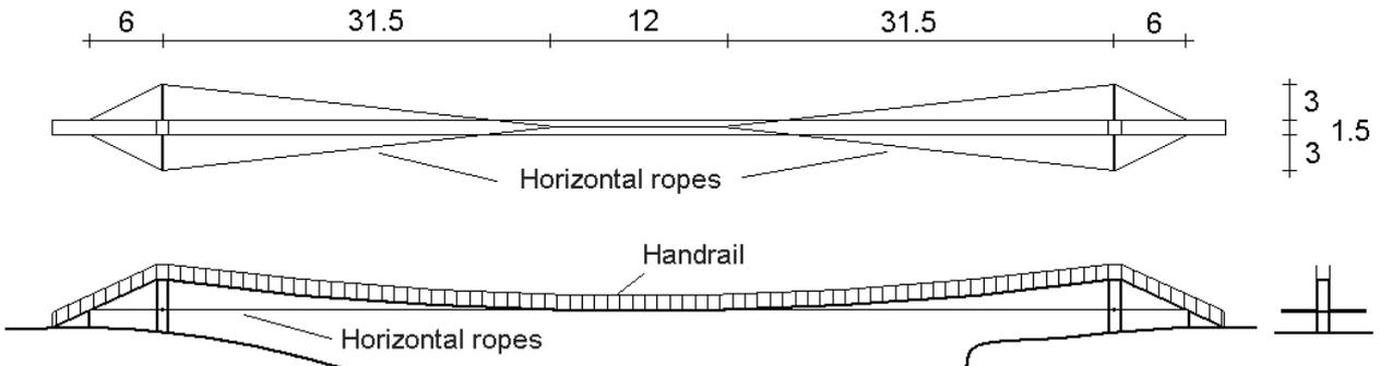
Fig. 3. View of footbridge A in Myślenice (dimension in meters)
