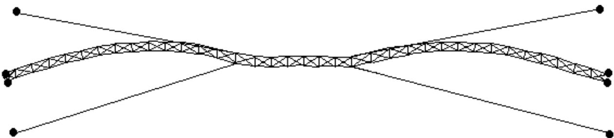
Fig. 7. I-st symmetrical vibration mode of footbridge A, plain view
