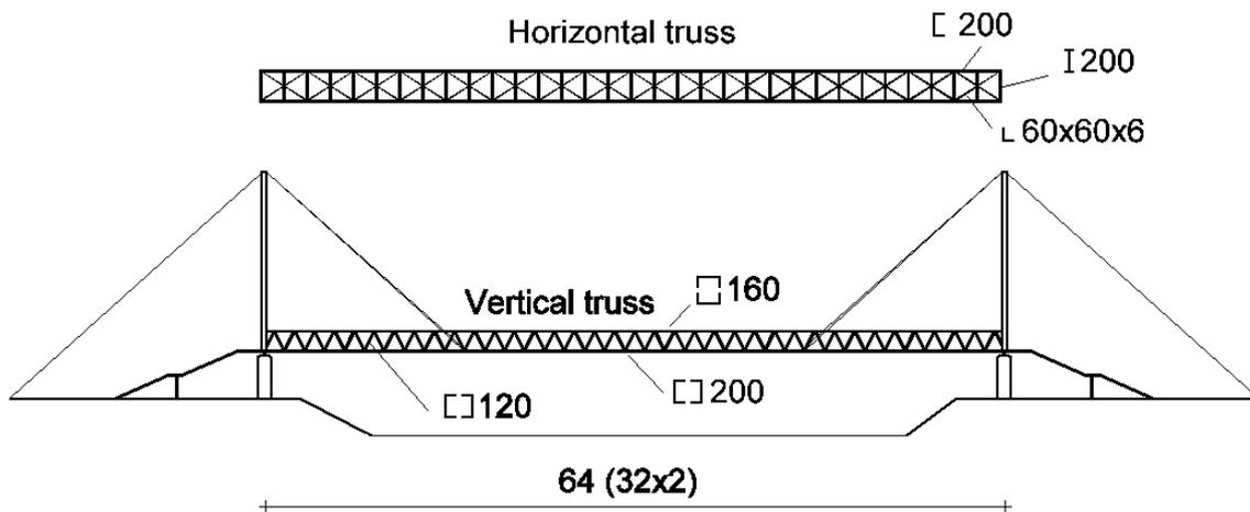
Fig. 6. View of footbridge D in Rzeszów (dimension in meters)
