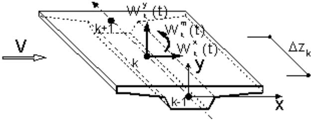
Fig. 2 A sector of span of bridge under wind load
